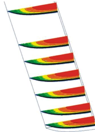
Fig. 7. Contour plots for primary velocities along the span of the channel for structured/boundary layer mesh
